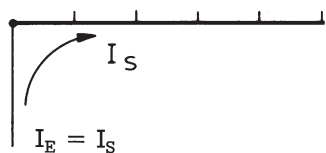
Feed in from the end of the busbar
